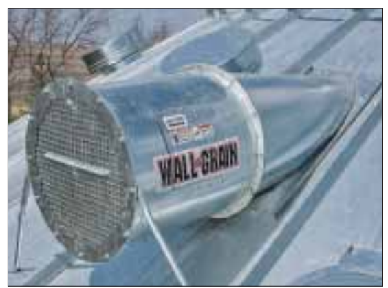
The Fast Dry method increases dryer efficiency by 20 to 30 percent. It quickens natural air drying in the bin by adding heat, allowing farmers to dry grain in seven days or less instead of weeks or months. | WALL GRAIN PHOTO
